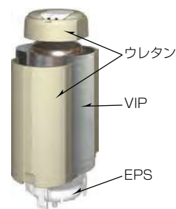
VIP : Vacuum Insulation Panel EPS : Expanded Poly-Styrene
