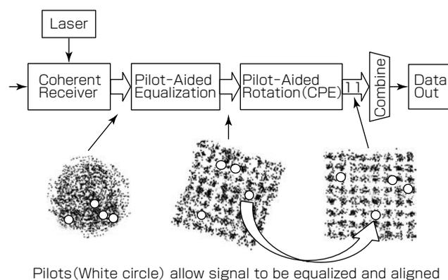
Fig. 3 Pilot-aided DSP for a single subcarrier
