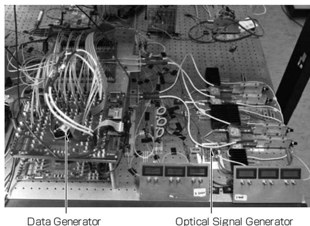
Fig. 2 Transmitter equipment
