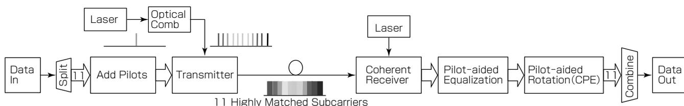
Fig. 1 Transmitter/Receiver Block Diagram
