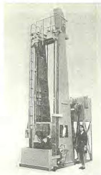
図9. 大形立形焼入装置 Vertical hardening equipment for long shaft.
