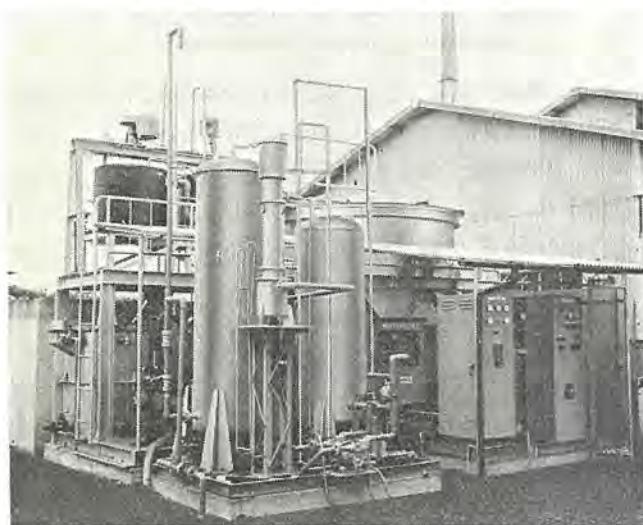
図 14. 凝沈+オゾンによる染色排水処理装置 Ozone treatment plant for dyeing waste water (Coagulating sedimentation + Ozonation).
