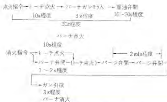
図 5. 個別バーナ点消火概要 Example of individual burner start stop sequence.
