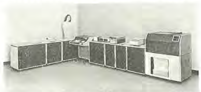
図 2.1 MELCOM 88 (拡張構成) MELCOM 88 office computer system (expanded configuration).
