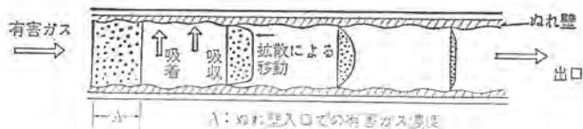
図 3.5 ぬれ壁小孔内での吸収、拡散によるガス濃度分布モデル Schematic distributions of gaseous concentration caused by absorption and diffusion in a holelet surrounded with wet walls.
