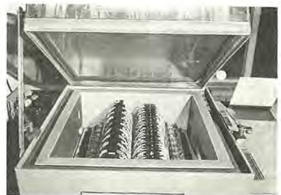
図 4.8 亜硫酸ガス中の接触信頼度試験状況 State of contact reliability test in the sulphurous acid gas
