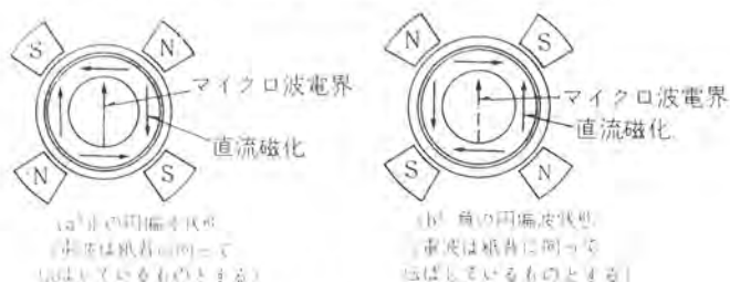
図 2.3 正と負の円偏波状態 Positive and negative circularly polarized states.
