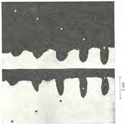
図 3.5 穴の断面と焦点ずれ (Al 1.6 J・印は焦点) Section of hole vs. shift of focal point.
