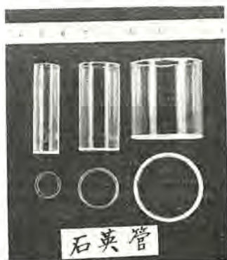
図 4.7 石英管 Quartz tube cut with CO 2 laser.
