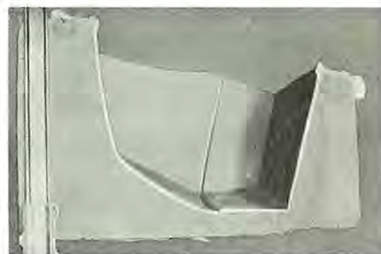
図 6.1 硫酸銅電鍍浴による電鍍層厚さ Thickness of electroformed copper with sulfate acid copper bath.
