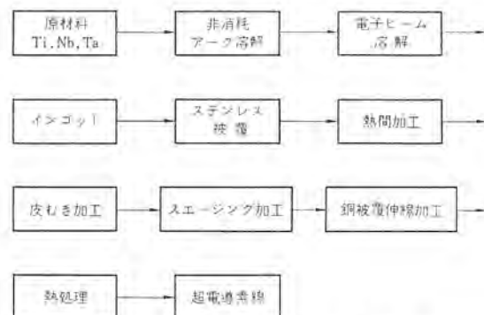
図 3.1 Ti-Nb-Ta 系超電導線の製造工程 Manufacturing process of superconducting Ti-Nb-Ta alloy wires.
