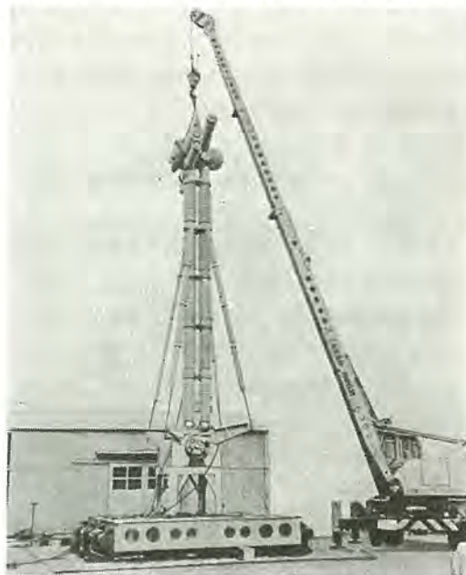
図 4.7 加振状況 Under shaking test of hyper high-circuit breaker.
