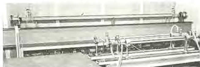
図 5.1 CO 2 レーザ装置の外観 (CO 2-300-44, -100-19) Exterior view of CO 2 laser equipments of type CO 2-300-44 and -100-19.
