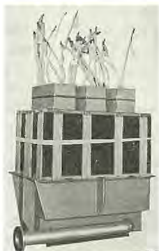
図 3.4 鉄心積み完了後の中身 Interior view after core assembly.
