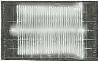
図 3.2 溶接中の溶接電流の変化 Amplitude variation of welding current during welding.
