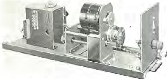
図 4.5 遅速自動平衡形指示計 Self-balancing indicator with slow balance speed.
