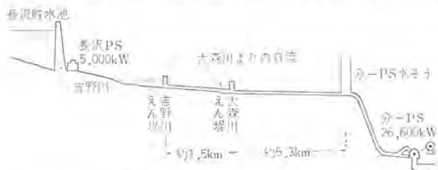
図3.1 長沢～分水第一発電所間水路図 Hydrographic sketch between Nagasawa and Bunsui power station No. 1.
