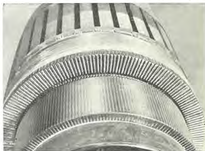
図 5.2 TIG 溶接ライザ Commutator with TIG welded riser.
