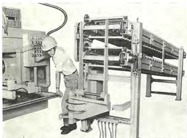
図 3.3 アクスルシャフト低ひずみ焼入装置 (供給装置付) Low strain hardening equipment of axle shaft (with feeding devices).
