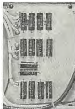
図 4.12 飽和・不感帯要素外観 Appearance of the limiter and dead zone element.
