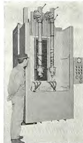
図 4.2 立て形 2 軸焼入装置 (コイル昇降形) Vertical type two shaft hardening equipment (coil being moved up and down).
