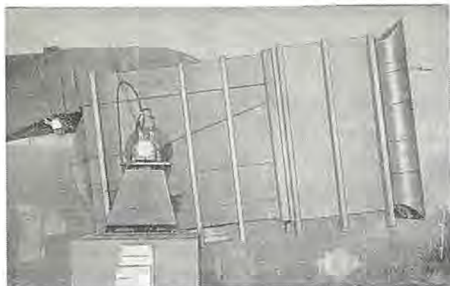
図 4.117 KC 形翼形押込送風機 Type KC airfoil blading forced draft fan.
