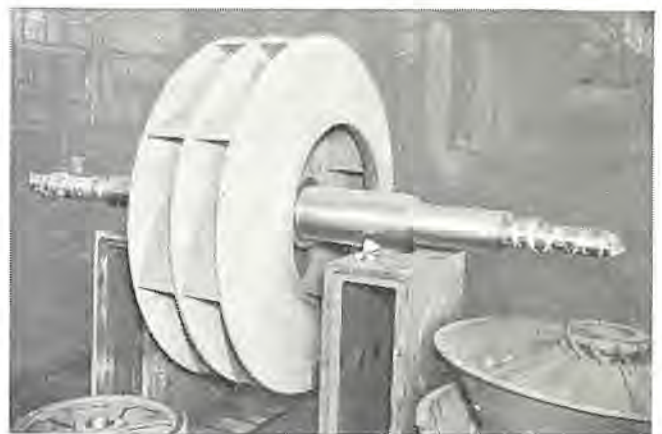
図 4. 116 KC 形翼形送風機扇車 Type KC airfoil blading fan runner.
