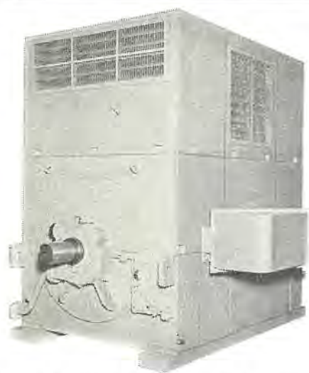
図 2.13 電発高砂納め給水ポンプ用U Line 形防滴保護形サイレンサ付き三相誘導電動機 3,600 kW, 6,600 V, 4極, 1,800 rpm Type U Line 3,600 kW 3 phase induction motor for a feed water pump of Takasago Thermal power station, the Electric Power Development Co.
