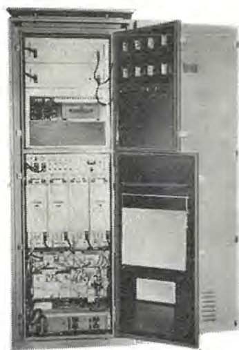
図 11.13 列車無線用新形無線電話中継機 Radio repeater for train radio telephone.
