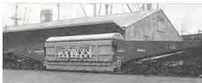
図 3. 1 240 t 積貨車で組立輸送中の関西電力姫路第 2 P/S 納め三相 510 MVA 超高圧変圧器 Three-phase 510 MVA extra-high voltage transformer being shipped on the 240 t schnabel car.
