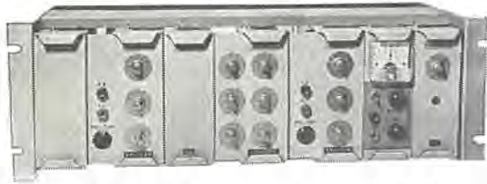
図4.83 接せん(栓)形工業制御用演算器他 Plug in type transistorized operational amplifier etc.
