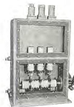
図 4.3 3 位置スイッチ内部構造 Interior view of three-position disconnecting and grounding switch.
