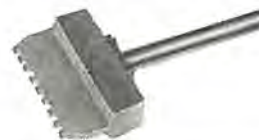
図 3.12 電極(ロータ3個同時加工用) Electrode for deburring of rotor (This electrode deburs three rotors simultaneously).
