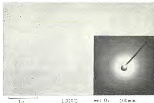
図 4.4 Si 酸化膜の透過 EM 写真および回折像 Fig. 4.4 Transmission electron microphotographs and electron diffraction pattern of silicon oxide film.
