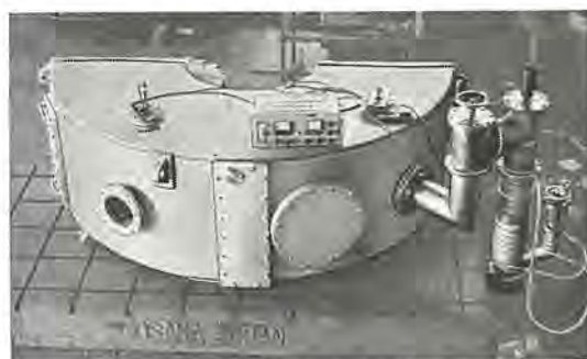
図 4.2 真空箱 ( r_0=75 cm) Fig. 4.2 Vacuum chamber of the r_0=75 cm air-cored beta spectrometer.
