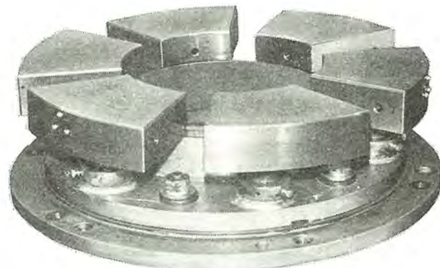
図 3.12 推力軸受の組立状態 Fig. 3.12 Assembling of thrust bearing.
