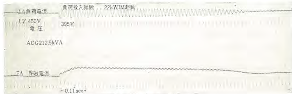
図 5.3 負荷投入試験 Fig. 5.3 Full load throwing test.
