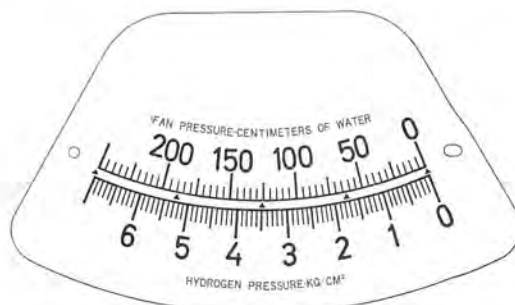
図 2.8 ガス・ブロウ連成圧力計目盛 Fig. 2.8 Dial of dual hydrogen pressure pneumatic transmitter and generator fan pressure gauge.
