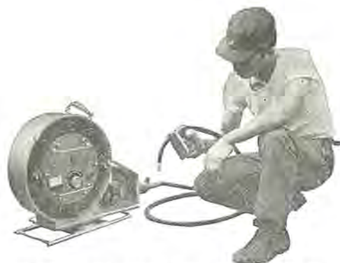
図 3.8 SA-400 形半自動溶接装置 Fig. 3.8 Type SA-400 semi-automatic arc welder.
