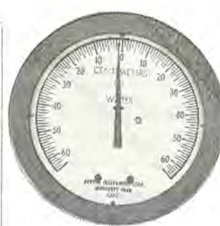
図 6.6 密封油差圧計 Fig. 6.6 Seal oil differential pressure meter.
