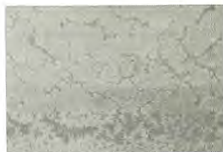
図 4. 3 E. C. Coating の顕微鏡写真 [ \times 400 ] Fig. 4.3 Photomicrograph electro-conducting transparent coating.
