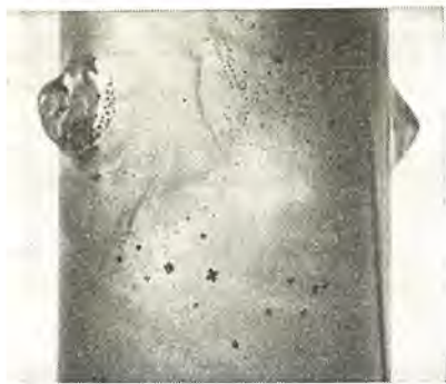
図 2.1 管壁上のヨウ素の結晶 Fig. 2.1 Iodine crystal deposits on the inner wall of the arc tube.
