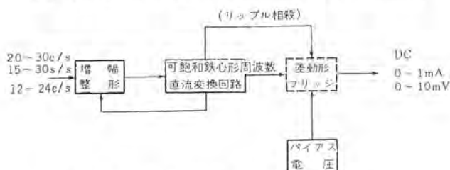
図 2.4 TM-R5 形受量器回路構成 Fig. 2.4 Block diagram of type TM-R5 receiver.
