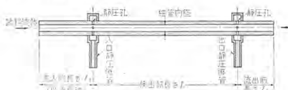
図 2.3 細管粘度検出器の静圧測定部 Fig. 2.3 Pressure tap arrangement of the capillary tube viscometer.
