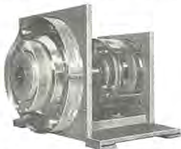
図3.3 グリス循環試験装置 Fig. 3.3 Testing device of circulation of ball bearing grease.
