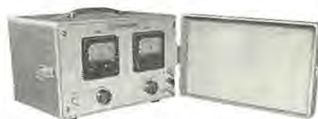
図5.3 テイ倍器調整用計器 Fig. 5.3 Measuring instrument of Varactor frequency multiplier.
