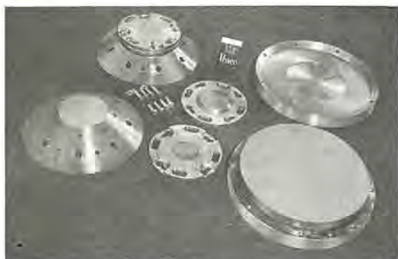
図 2.5 磁極片 Fig. 2.5 Convertible pole-pieces.
