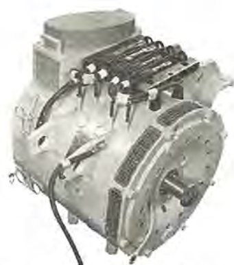
図 4.2 MB-3054-B 形主電動機外観 Fig. 4.2 Type MB-3054-B traction motor.
