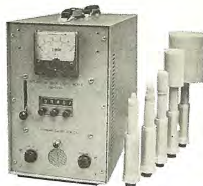
図 19-18 電離箱式線量計 Integrating dose rate meter employing ionization chambers.
