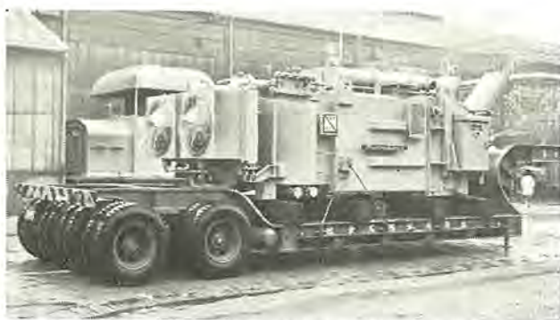
図 2-3 関西電力納め 140 kV 90 MVA 移動用変圧器 (一相分) One phase of 140 kV 90 MVA mobile transformer bank for the Kansai Electric Power Co.
