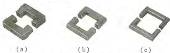
図 18-9 小形化の例 Reduction in the size of flyback transformers.
