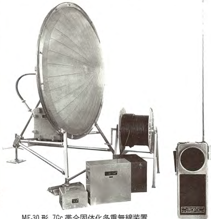
ME-30 形 7Gc 帯全固体化多重無線装置 Type ME-30 all solid state radio equipment in 7 Gc band.
