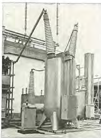
図 2-23 大容量短絡試験設備でシャ断試験中の 300kV 2,000A 20,000MVA GW 形油 シャ断器 Type "GW" oil circuit breaker rated at 300kV 2,000A 20,000MVA under interrupting tests at high power laboratory.
