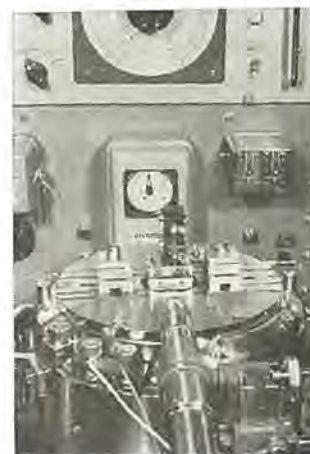
図 18-14 パネ用薄板・線の疲れ試験装置 Fatigue testing equipment for thin plate and wire spring materials.
