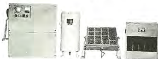
図 11-28 無線雨量観測局装置 Telemetering equipment of rain full observing station.
