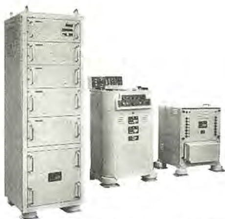
図 12-4 D 形 M.T.T., RPPI, RPPI 用電源外観 Front view of type D MTT, RPPI, power supply unit for RPPI. (from left to right)
