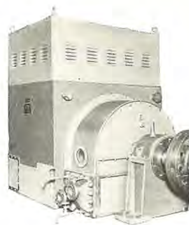
図 5-1 新南極観測船“ふじ”納め全閉内冷形自動交流発電機 3×625 kVA 450V 10P 720 rpm 625 kVA 450V 10 P 720 rpm totally enclosed inner cooled self excited AC generator for antarctic expedition ship.
