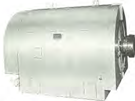
図 1-8 東京電力納め強圧通風機用 2,200 kW, 4,000 V, 50 c/s, 6 極, 1,000 rpm 全閉外扇形屋外誘導電動機 Type MKT-W three phase induction motor for a forced draft fan delivered to the Tokyo Electric Power Co.
