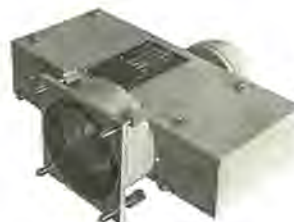
図 11-16 ME-7 A 02 形, 7 Gc 帯 FPU 用 TDA Type ME-7 A 02, 7 Gc band TDA for field-pick-up equipment.
