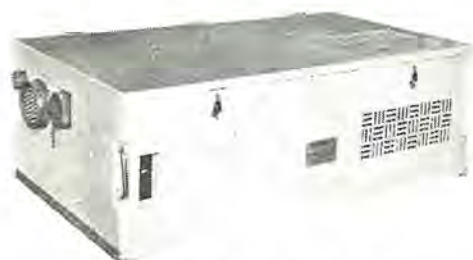
図 6-14 論理照査回路箱 Case of speed checking and logic apparatus.
