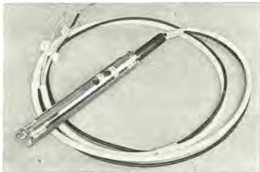
図 1.1 微小電極用前置増幅器外観 Fig. 1.1 Outside view of the microelectrode preamplifier.
