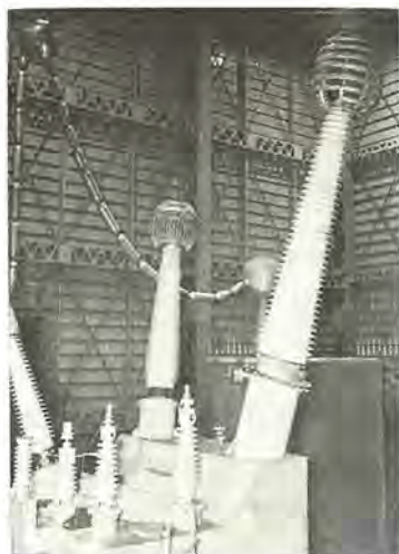
図 5.2 試験中の超々高圧短絡変圧器 Fig. 5.2 Extra high voltage transformer under testing in the high voltage laboratory.
