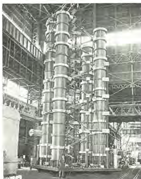
図 2.1 4,000 kV 600 kJ 衝撃電圧発生装置 Fig. 2.1 Exterior view of 4,000 kV 600 kJ impulse voltage generator.
