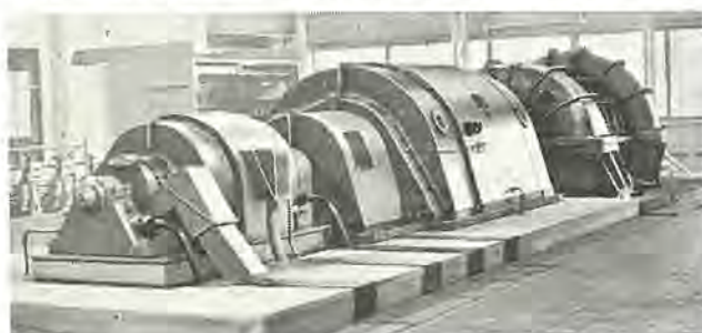
図 1.1 高炉ブロワ駆動用9,200 kW 2極同期電動機 Fig. 1.1 A 9,200 kW 2-pole synchronous motor for driving a blower of blast furnace.
