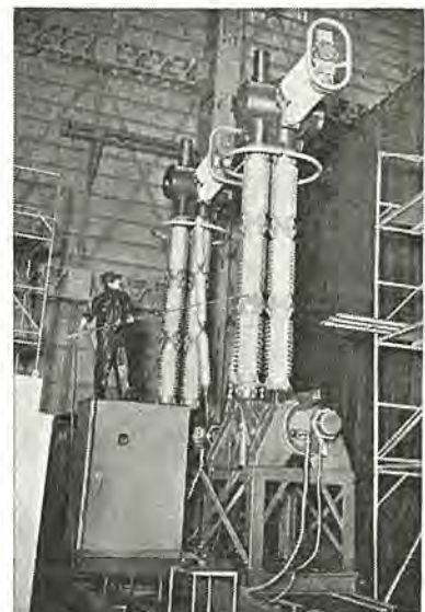
図 4.2 300 kV ガスシヤ断器の汚損スプレー状況 Fig. 4.2 300 kV, 25,000 MVA, SF 6 circuit breaker in spraying for contamination test in high voltage laboratory.
