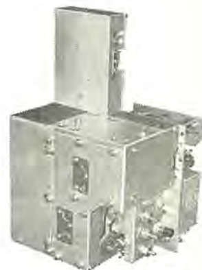
図 4.4 自動同調部 Fig. 4.4 Automatic tuning control and mechanical drive subassembly.
