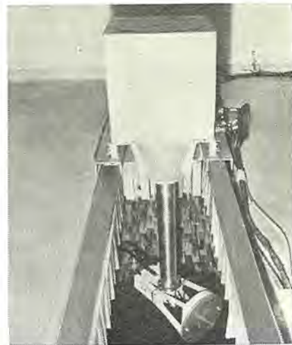
図 4.22 送受波器回転機構 Fig. 4.22 Transmitter-receiver rotating mechanism.
