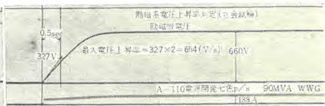
図 5.7 励磁系頂上電圧測定 Fig. 5.7 Measurement of the ceiling voltage of the excitation system.
