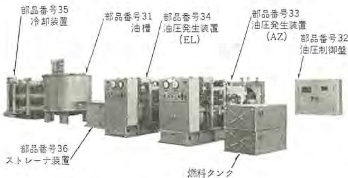
図 4.11 油圧発生装置 Fig. 4.11 Arrangement of hydraulic power source.
