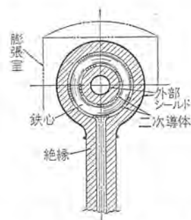
図 4.1 大電流用変流器の新形絶縁の断面図 Fig. 4.1 Cross section of new insulation for a large current.
