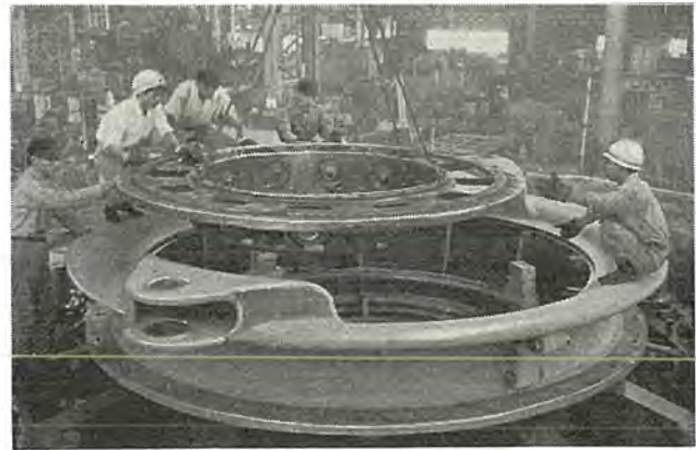
図 5.9 工場組立中の軸受ささえ Fig. 5.9 Bearing support under assembling at the factory.
