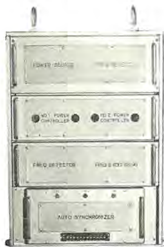
図 6.1 XPF 形自動負荷分担装置 Fig. 6.1 Type XPF automatic power and frequency controller.
