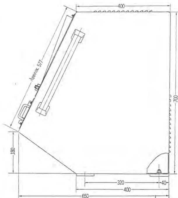
Fig. 3.6 (b) Outline dimensions of monitor console.
