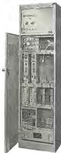
図 4.1 送信架 Fig. 4.1 Transmitter of mobile station.
