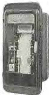
図 10.7 MZ 形印字式記録積算計器 Fig. 10.7 Type MZ print recording integrating meter.
