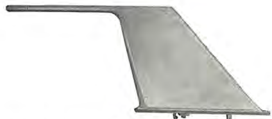
図 7.10 列車用架線電圧検知・VHF 帯無線共用アンテナ Fig. 7.10 Blade antenna for common use in trolley wire voltage detectors and VHF radiotelephone equipments for trains.
