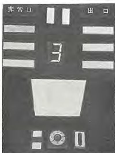
図 11.7 EL ランプの応用例 Fig. 11.7 Applications of EL lamp, meter dial, sign board, numerical indicator, switch plate, night light.
