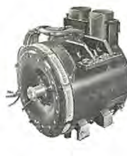
図 5.5 小田急回生車用 MB-3095-AC 形主電動機 Fig. 5.5 Type MB-3095-A C traction motor for OER (Odakyū) car provided with regenerative brake.
