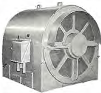
図 3.7 全閉外扇 300kW MKT 5614 6,000 V 50 c/s 8P 750 rpm Fig. 3.7 MKT 300 kW totally enclosed fan cooled motor.
