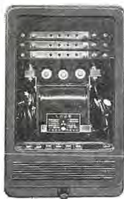
図 2.7 正相分 0/1 器式入力装置 Fig. 2.7 Typical input circuit device consist of positive sequence filter and saturation transformer.
