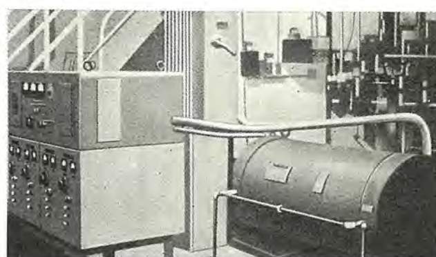
図 11.1 20,000 c/s 高周波発電機の並列負荷運転 Fig. 11.1 20,000 c/s high frequency generator in parallel loading.
