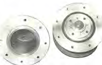
図 3.1 小形火炎逸走実験器 Fig. 3.1 A small size testing device of communicating the internal inflammation to the external explosive gas.
