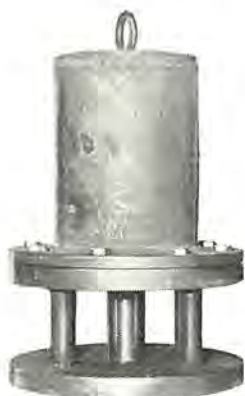
図 3.1 小形火炎逸走実験器 Fig. 3.1 A small size testing device of communicating the internal inflammation to the external explosive gas.
