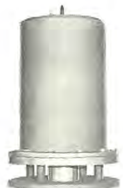
図 3.3 大形火炎逸走実験器 Fig. 3.3 A big size testing device of communicating the internal inflammation to the external explosive gas.
