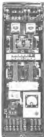
図2.14 KKS-2形特性距離継電器外観 Fig. 2.14 View of type KKS-2 square characteristic distance relay.
