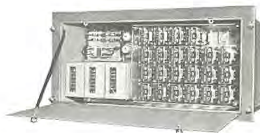
図 5.1 論理部引出し外観 Fig. 5.1 Outside view of a logic relay box.
