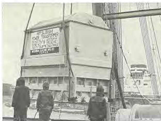
図 7.1 船積中の 145 MVA 変圧器 Fig. 7.1 145 MVA transformer being lifted for shipping.
