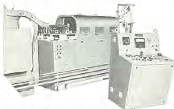
図 4-9 鍛造用誘導加熱装置 (3 kc 300 kW) 3 kc 300 kW induction heater for forging.
