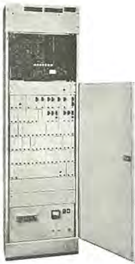
図 11-63 列車運行ダイヤ自動 記録装置 (A 装置) Railway traffic supervising equipment. (A denice)
