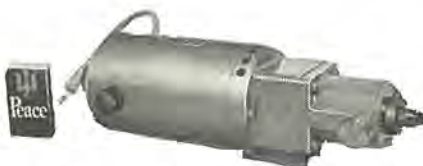
図 4-121 FB 形整流子電動機 200 W, 100 V, 50/60 c/s, 10,000 rpm (小形工 作機用) FB type single phase commutator motor for small machine tool.
