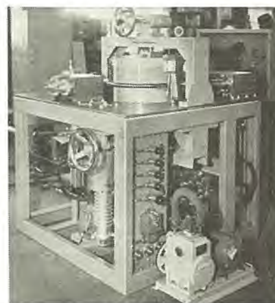
図 20-32 立体収束質量分析計 Two-direction focussing mass spectrometer main body and pumping system.
