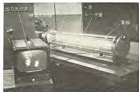
図 20-17 He-Ne ガスレーザ装置 The experimental setup of He-Ne gas laser and a radiation pattern.
