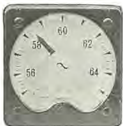
図 14-1 変換形周波数計 Transducer type frequency meter.
