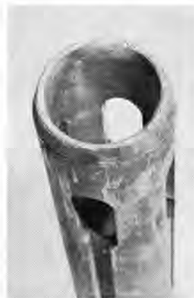
図 5.8 33 kA を 30 回シャ断、3 回投入した可動接触子 Fig. 5.8 Photograph showing the moving contact after 30 interruptions and 3 closings of 33 kA rms.
