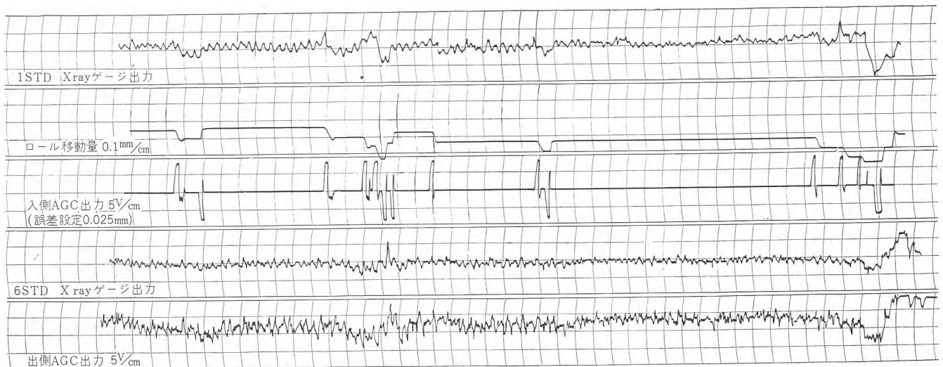
図 6.2 AGC 压下制御・張力制御実記録 Fig. 6.2 Practical operation characteristics of roll screw down control AGC system.
