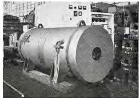
図 4-123 千代田鋼管納め 250 kVA 800 V 10,000 c/s 3,000 rpm 高周波発電機入力 330 kW 3,300 V 三相 50 c/s 2 極誘導発電機駆動 High frequency generators 250 kVA, 800 V 10,000 c/s 3,000 rpm, with driving induction motor, 330 kW, 3,300 V 3 phase, 50 c/s 2 poles.
