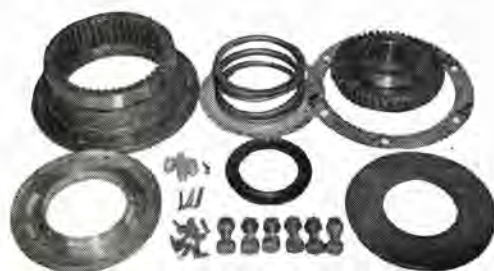
図 7-11 WN-560-BK 形ギヤカップリング部品 Parts of type WN-560-BK gear coupling.
