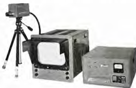
図 12-36 IT-5 形産業用テレビ装置 Type IT-5 industrial TV equipment, left to right; camera, control monitor and power supply.
