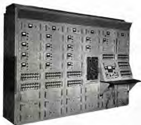
図 12-14 EA-7105 形座標変換器 Coordinate transformation computer. (type EA-7105)
