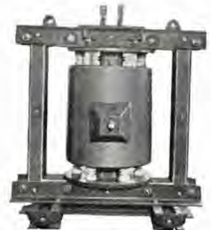
図 2-11 単相 65kVA 10 分間定格 60c/s 発電機中性点接地用 A 種絶縁乾式変圧器 17,200V BIL 120kV/240V Single phase class A insulation dry type transformer for grounding a neutral point of generator 65kVA 10min rating 17,200 V BIL 120 kV/240 V.
