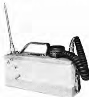
図 11-4 WT-5 形 VHF/FM 携帯無線機 Type WT-5 VHF/ FM portable radio equipment.
