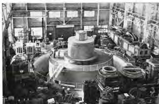
図 1-26 滝発電所納め 50,000 kVA 150 rpm 50,000 kVA AC generator for Taki Power Station.
