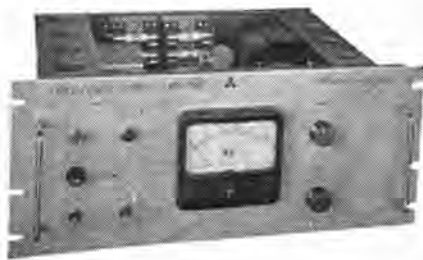
図 14-30 高圧安定化電源 Stabilized high voltage supply ND-1522.
