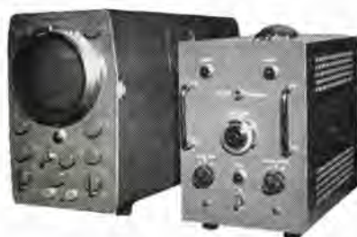
図 12-23 FD-5C 形超音波探傷機と自動警報装置 FD-5C Ultrasonic flaw detector (left) and automatic alarm equipment. (right)
