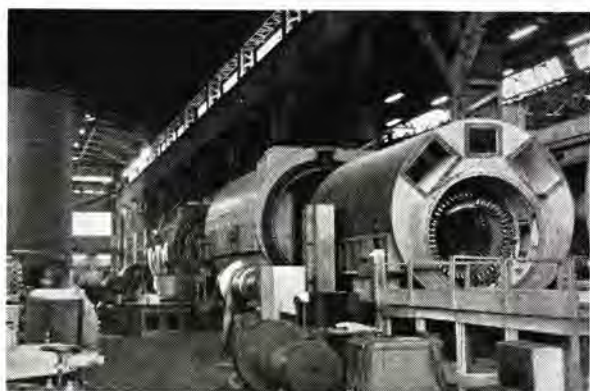
図 1-2 工場で製作中の電力用大容量タービン発電機群 Large capacity turbine generator group for electric power use under construction at the factory.
