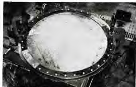
図 19-22 大変形薄肉円板の応力測定 Stress measurement of circular thin plate under large deflection.
