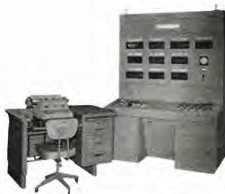
図 12-9 MELDAP-5712 高落差水車試験用計測盤 MELDAP-5712 for high head hydraulic turbine testing.
