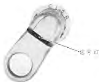
Fig. 4.11 Construction of type NT-2 circuit breaker.
