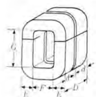
Fig. 3.2 Square type three phase unit.
