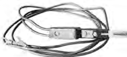
図 7.4 CT 回路電流測定用テストプラグ Fig. 7.4 Test plug for secondary circuit current measurement of current transformer.
