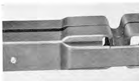
図 2.12 積層ツナギ Fig. 2.12 Welded laminate joint.
