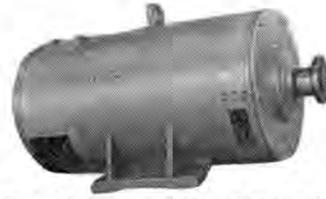
図 1-23 関西電力納め単相交流発電機 10kVA 単相 200V 60c/s 6 P 1,200 rpm 始動機励磁機兼用 10 kVA single phase AC generator for combined use as starter and exciter for Kansai Electric Power Co.
