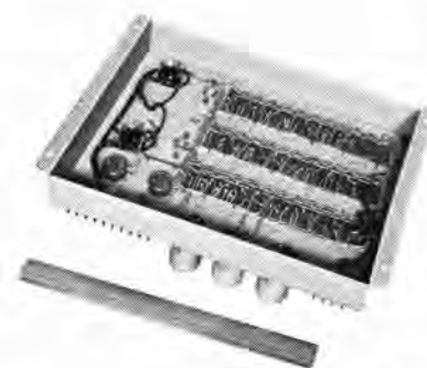
Fig. 3.3 Transistor relay panel (step feed device for drill head)
