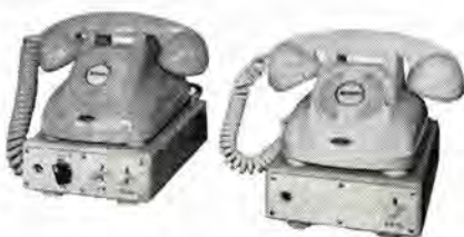
図 3.7 移動局超短波無線送受信架 Fig. 3.7 UHF transmitter and receiver bay of movable station.
