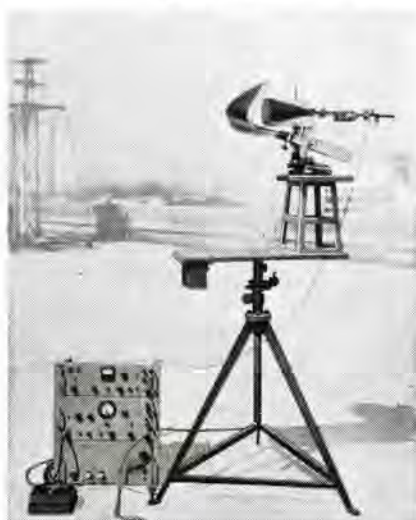
Fig. 4.1 Arrangement for measurement of power transmission coefficient.
