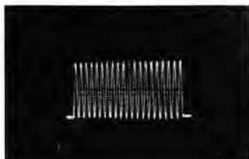
図 5.6 2,000 c/s 正弦波 Fig. 5.6 Sine wave of 2,000 c/s circle test.
