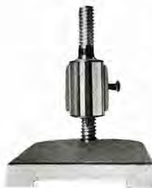
鉄心形差動変圧器 Core type differential transformer.
