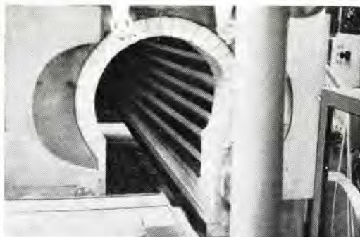
大形真空焼鈍炉加熱部 Large vacuum annealing furnace.
