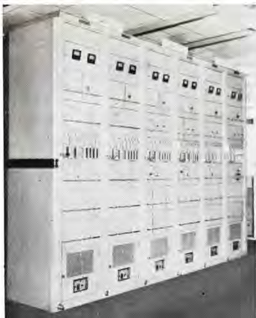
TZ-2 形 ARQ 端局装置 Type TZ-2 electronic 4/2 channel multiflex ARQ telegraph terminal.
