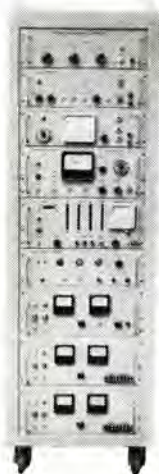
コロナ測定装置 Corona measuring equipment.
