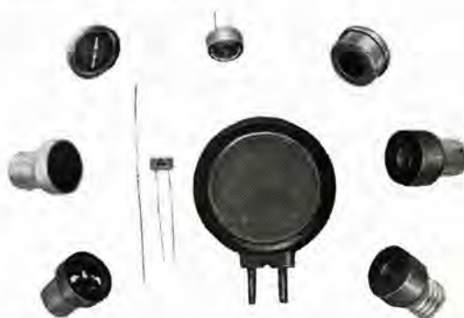
種々の形式の硫化カドミウム光導電セル Various types of CdS photoconductive cell.
